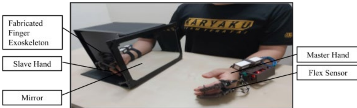
Figure 7: System integration of flex sensor from arduino circuit and fabricated finger exoskeleton in mirror therapy.
