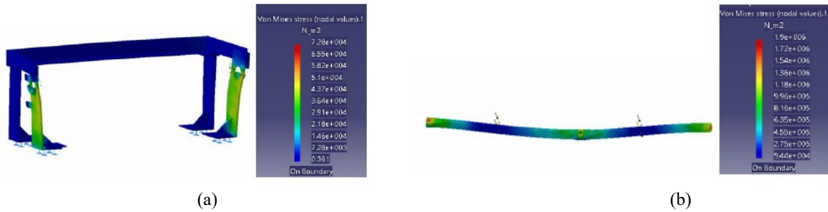
Figure 8: Finite Element Analysis on another selected part of portable STT device, (a) Leg structure (b) Von Shaft.
