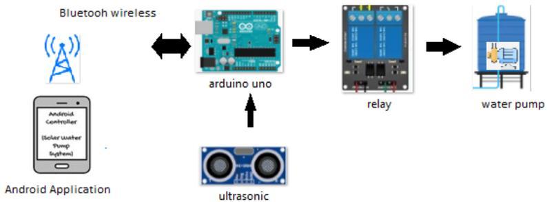
Figure 1: The controller system using Arduino UNO and connected with Bluetooth system
