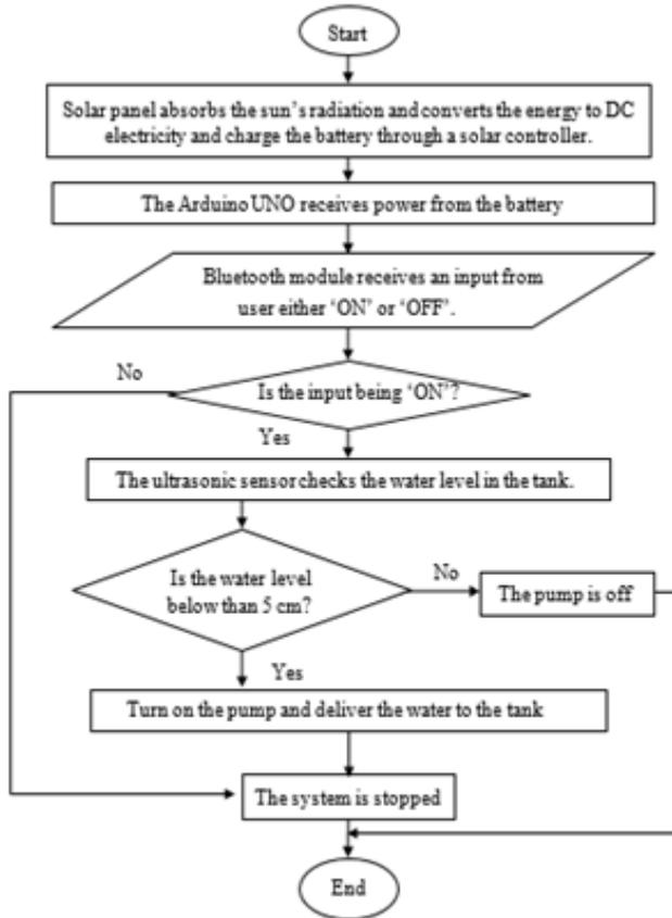
Figure 3: Flowchart of the water pump system
