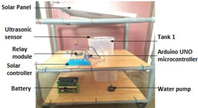
Figure 4: The prototype of the water pump system
