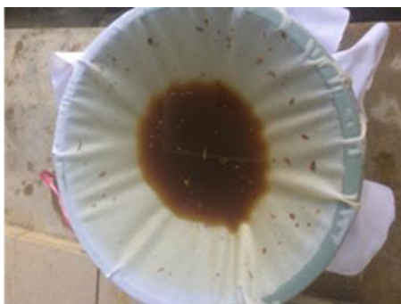
Figure 2: Sample photograph of the impurities after first time filtering the WCO.
