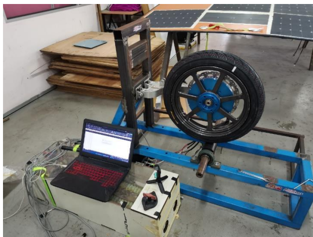
Figure 7: Testbench assembly hooked up to monitoring software
