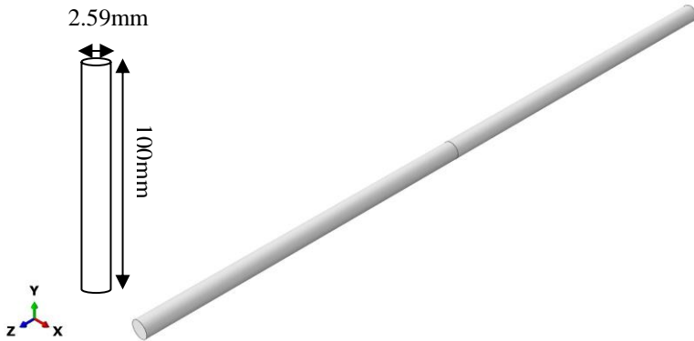
Figure 2: The dimension of the 3d printing filament
